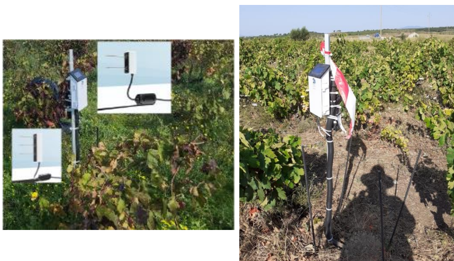
Figure 5. Soil moisture dataloggers and sensors installed in Roses (left) and Espolla (right)
