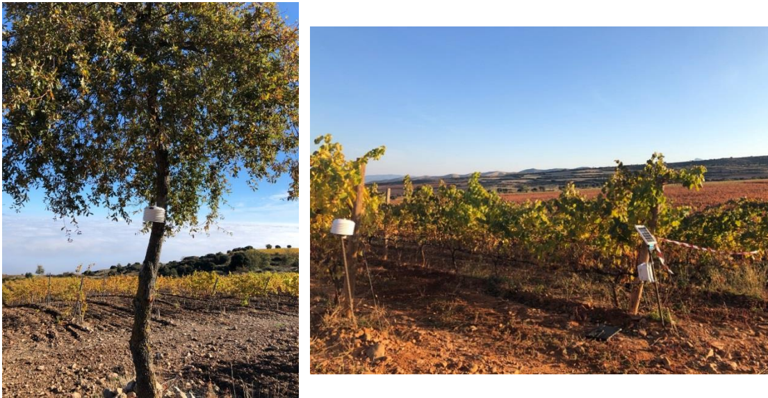
Figure 12. Air temperature and relative humidity sensors HOBO Logger installed in (left) Clavijo site (San Prudencio winery) and (right) Tudelilla site (Vivanco winery), La Rioja.
