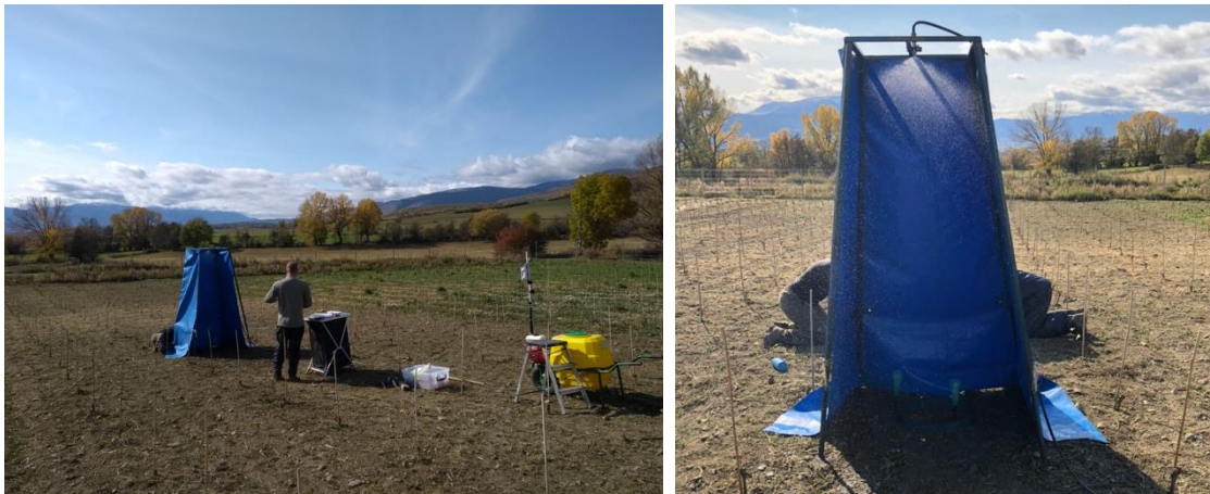
Figure 9. The rainfall simulator used during the experiments in Llivia (Catalonia): general view (left), simulator at work (right).
