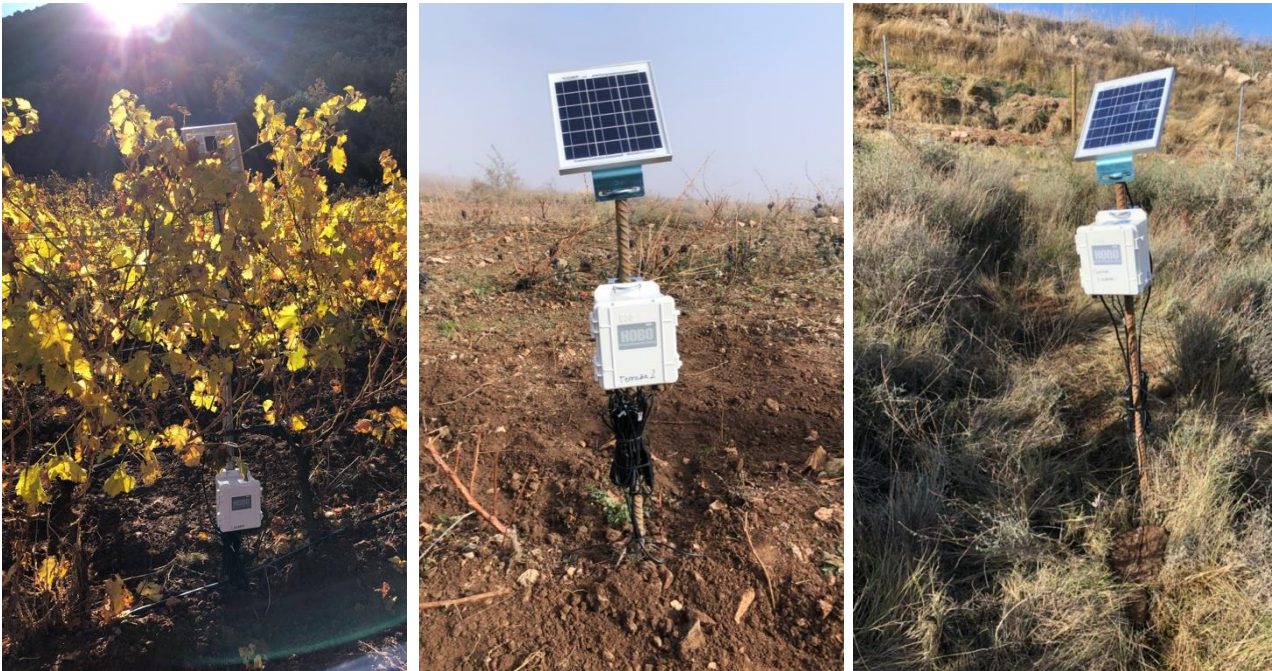
Figure 2. Soil moisture sensors and dataloggers in Clavijo (San Prudencio winery), La Rioja, in the hillside plot (left), terraced plot (middle) and hillside control plot (right).
