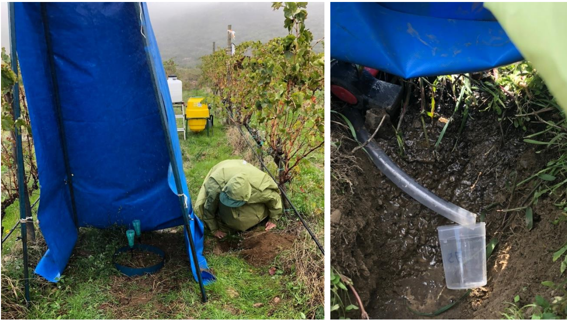
Figure 10. Collecting water samples during a rainfall simulation in Roses (Catalonia).
