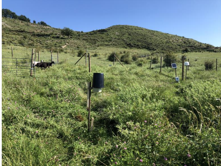
Figure 13. Pluviometer, temperature sensor and soil moisture sensors in San Román experimental site.
