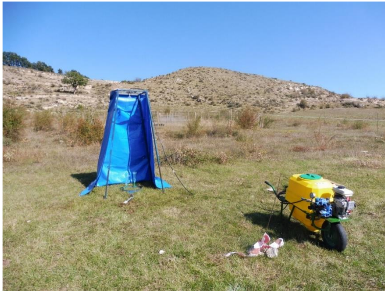
Figure 10. The rainfall simulator used during rainfall simulation experiments in San Román de Cameros (La Rioja).
