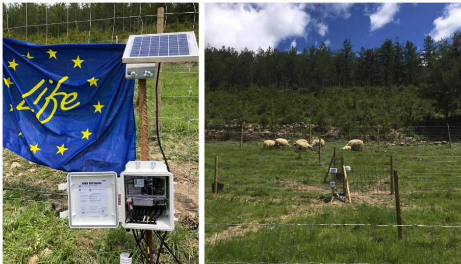
Figure 3. Soil Humidity (detail on the left side) and Termometer/Hygrometer dataloggers installation in La Garcipollera experimental plots.
