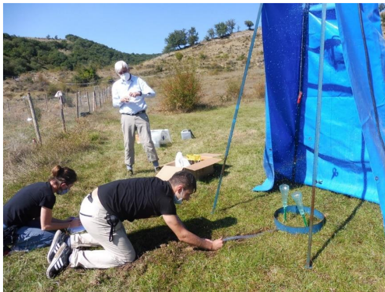
Figure 11. Collecting water samples during a rainfall simulation experiment in San Román de Cameros (La Rioja).
