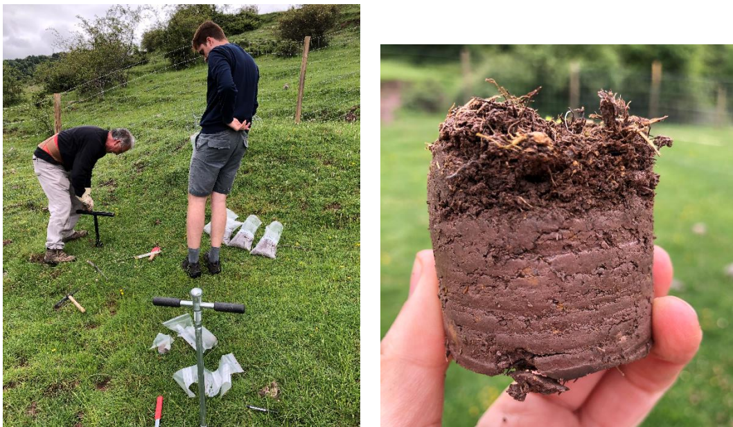
Figure 3. (a) Soil sampling in San Román (Calcareous soils), and (b) detailed undisturbed soil sample.
