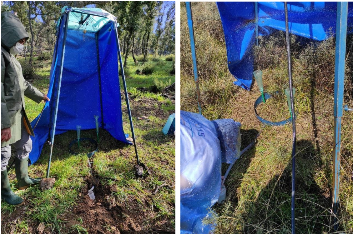
Figure 17. Left: The rainfall simulator used during the experiments in Requesens (Catalonia). Right: Collecting water samples during a rainfall simulation in La Garcipollera (Aragón).
