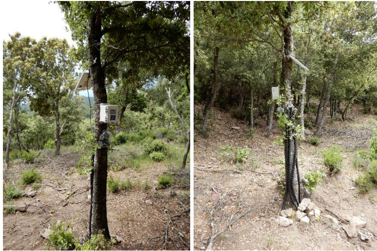
Figure 8. Soil moisture dataloggers and sensors installed in Requesens experimental plots (Catalonia).
