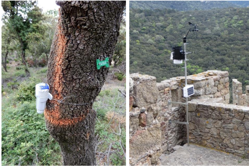
Figure 19. HOB0 Logger (left) and weather station (right) installed in Requesens (Catalonia).
